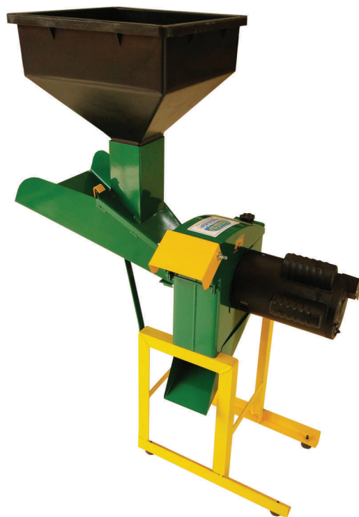
B 609 Compacta (Fornecida com motor 3 cv)
